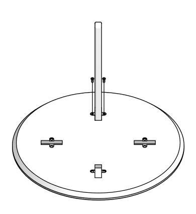
Insert Bolts through block into Table Top and hand thread in. Repeat Step 1 & 2 to attach remaining legs. Use provided Allen Wrench to securely tighten all bolts.
