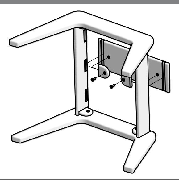
Place Slats over Braces by fitting groove track cut out with long edge of the Brace. Align threaded holes in Slats with pocket cut outs in Braces. Place Blocks G into pocket cut outs and insert bolts through the blocks into threaded holes and finger tighten.
