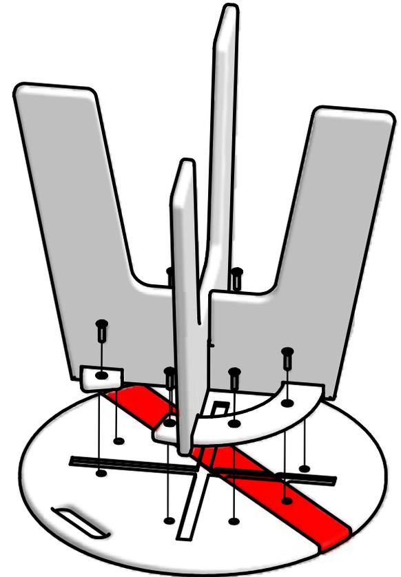
Align Edges of Legs with groove track cut outs of Top. Insert bolts through the Blocks into the Tops threaded hole inserts and finger tighten. Blocks may need to be adjusted to align holes.
