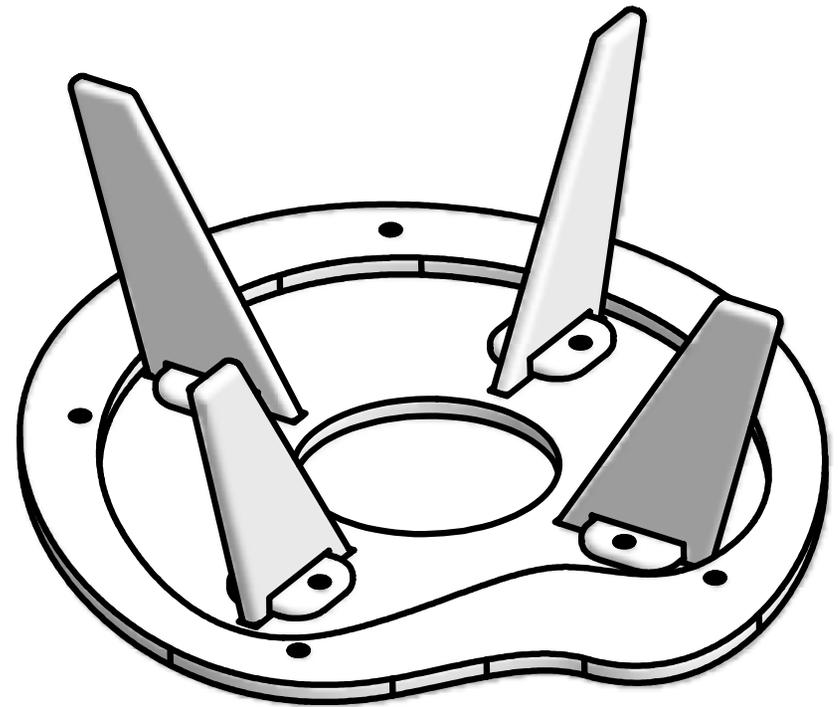
Repeat Step 1 to attach remaining legs. Use provided Allen Wrench to securely tighten all Bolts.
